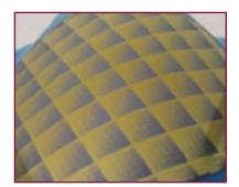
Si: diameter: 3 in to 200 mm; thickness: 50-725 µm
